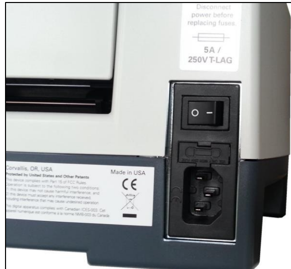
Shows the power module in the back of the embosser
